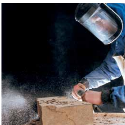
Photograph 8 Blowing off stone debris. Using the pneumatic exhaust to blow off stone debris creates a large fine stone dust cloud. This is reduced by soaking stone and keeping it damp but better still would be to vacuum or carefully brush off debris
