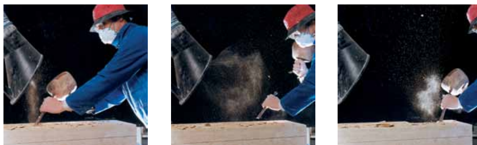
Photograph 6 Hand chiselling and captor hood exhaust ventilation. Sequence of three photographs shows stonemason working within the hood capture zone, partially within it and well outside it. Dust control is only effective when work takes place within capture zone (see Figure 14).
