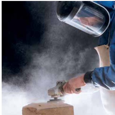
Photograph 4 Polishing. Polishing creates fast moving radial jets of dust-laden air which are difficult to control (also see Figure 10)
