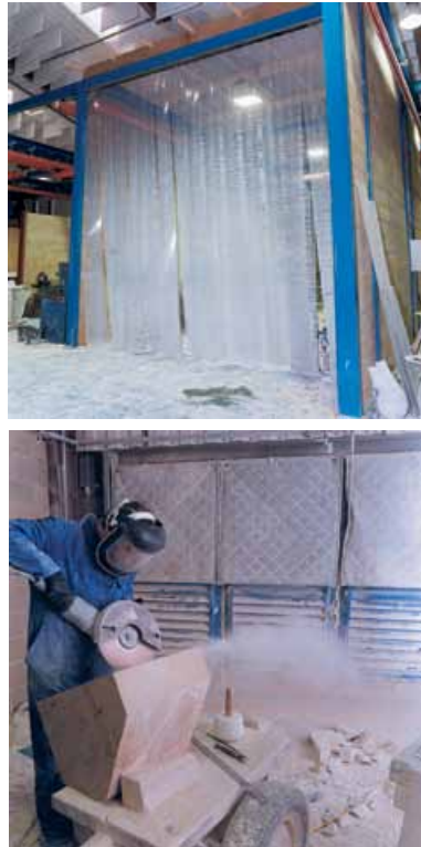
Photograph 5 Segregation of dusty processes. Figure 12 shows segregation in diagrammatic form and these two photographs show practical ways of segregating power tool work from less dusty stonemasonry processes.
