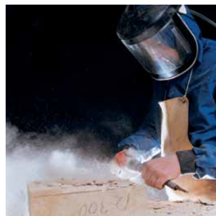
Photograph 8 Blowing off stone debris. Using the pneumatic exhaust to blow off stone debris creates a large fine stone dust cloud. This is reduced by soaking stone and keeping it damp but better still would be to vacuum or carefully brush off debris
